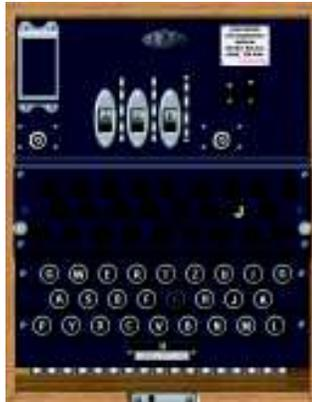
▲ This Enigma Simulator both looks and works like the famous WWII electromechanical cipher machine.
